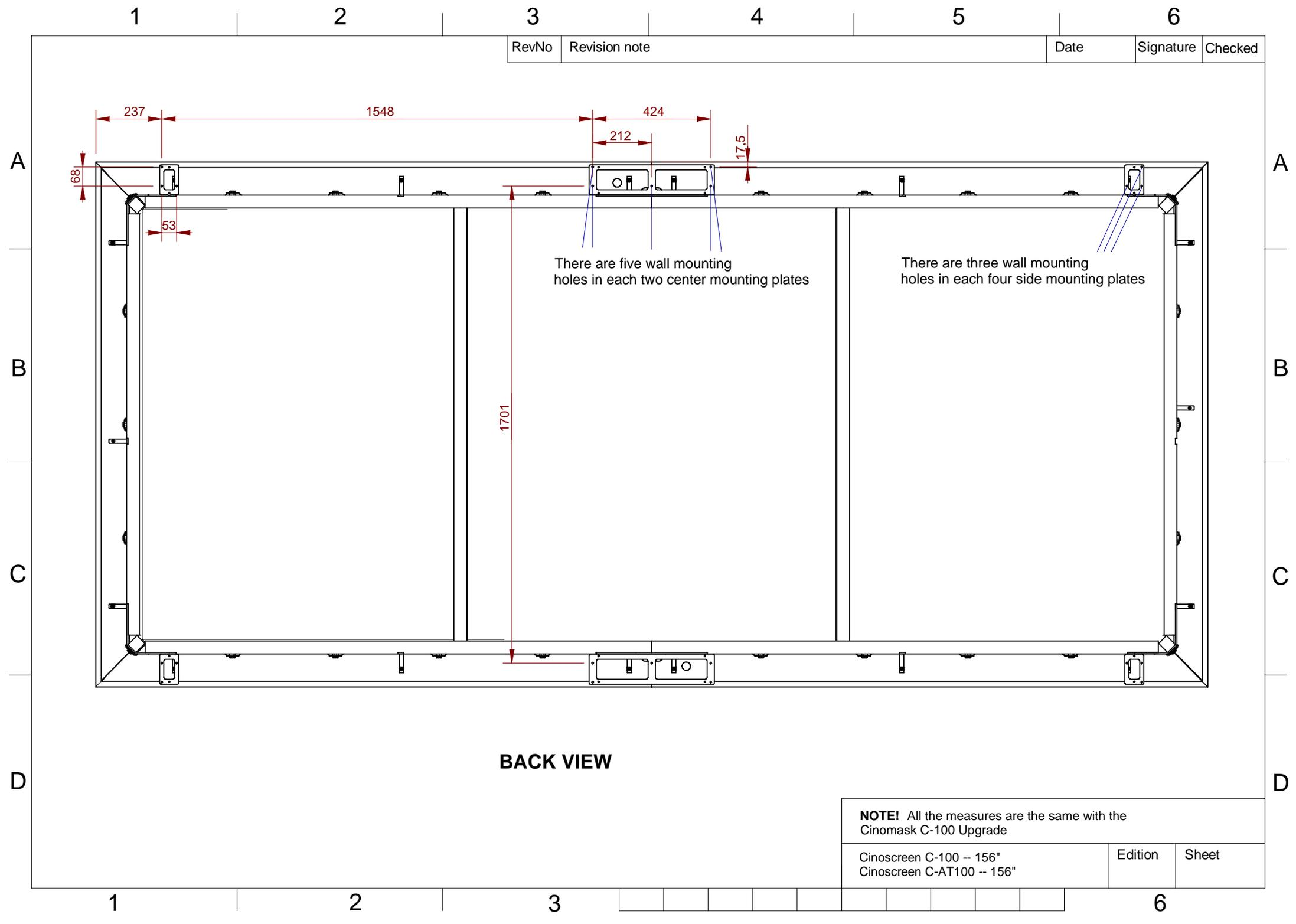
There are five wall mounting holes in each two center mounting plates
